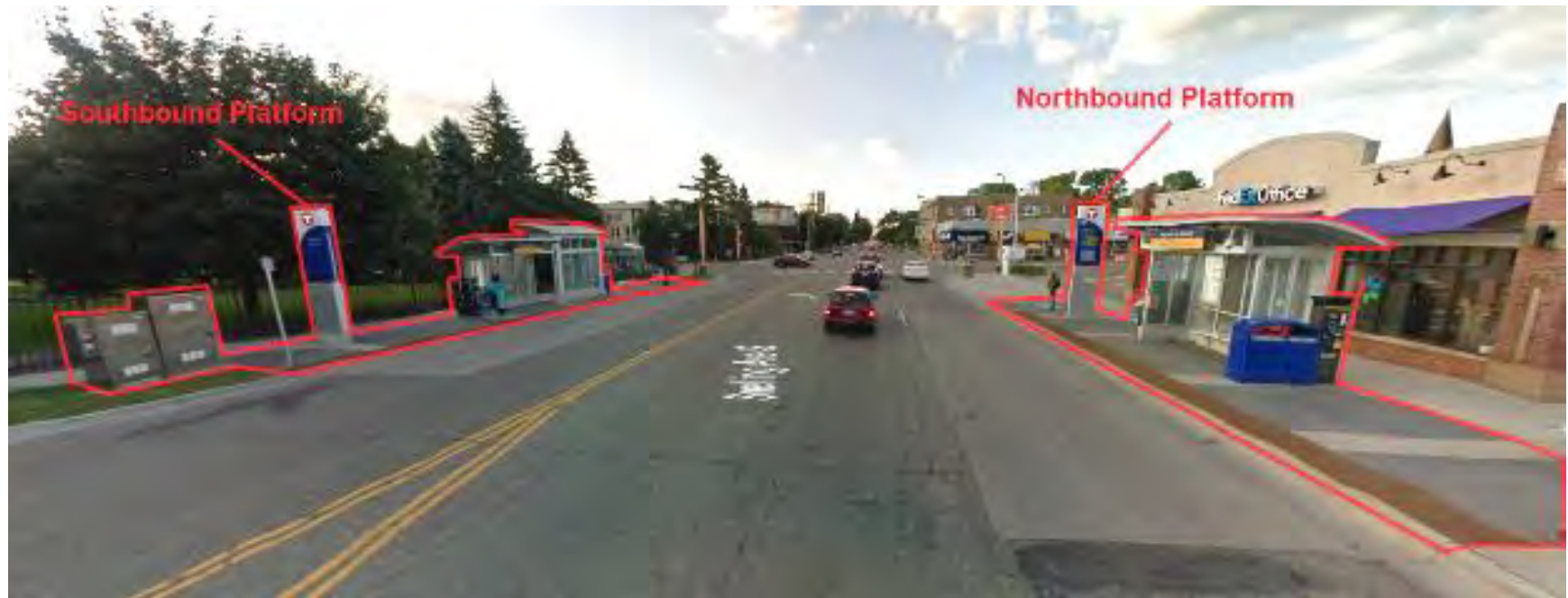
Typical BRT station with two directional platforms.
