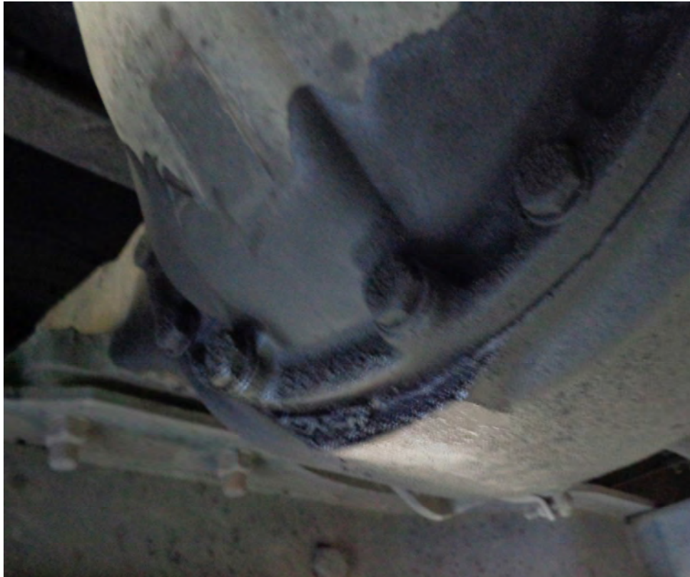
Bus 1205: Differential Gasket Leaking
