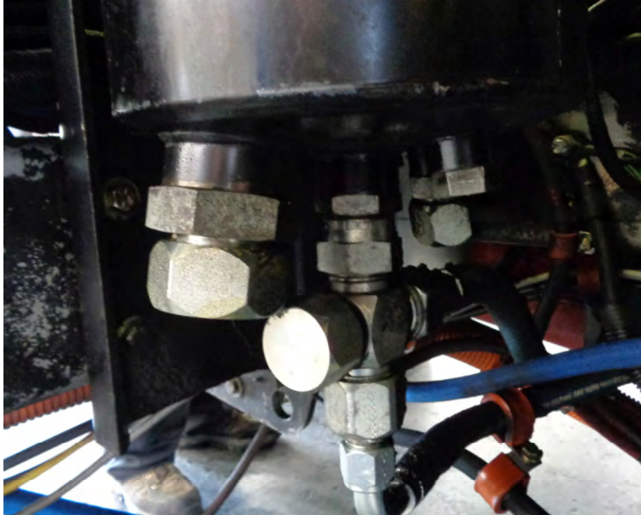
Bus 1005: Hose Leak at Hydraulic Reservoir
