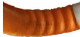
Figure 4-24, Not Acceptable Cable Puckering
