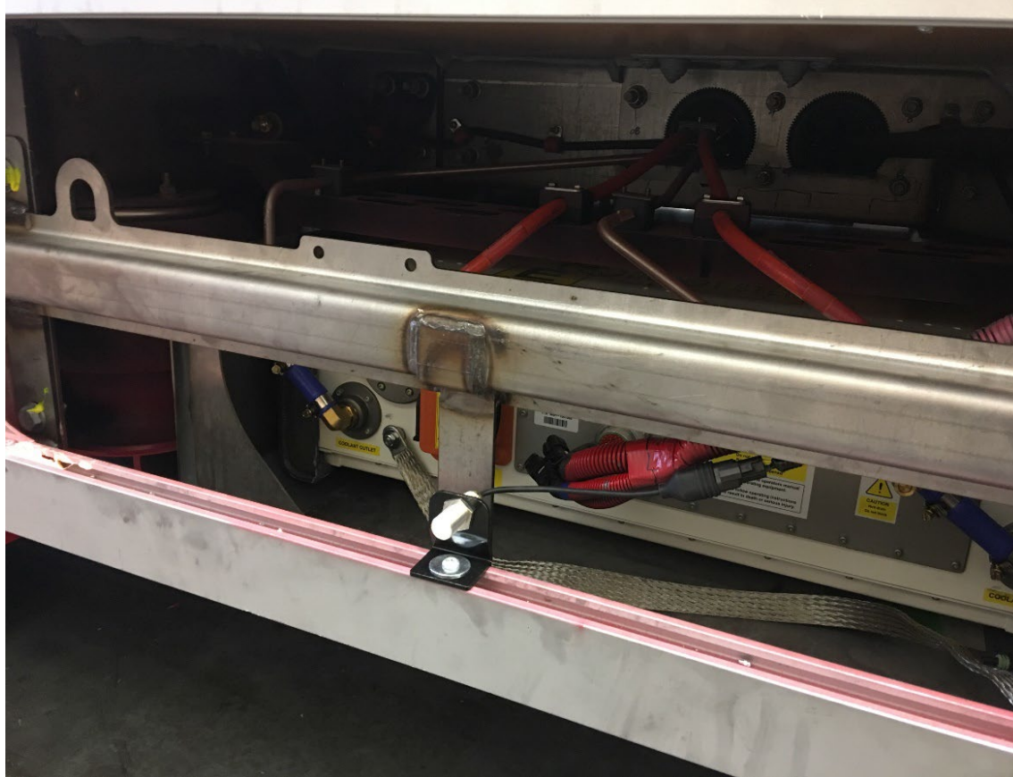
Curbside: Chassis Battery Access Body Panel Interlock Location
