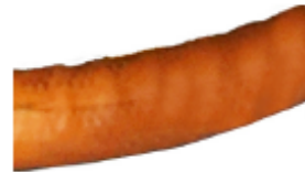
Figure 4-23, Acceptable Cable Puckering
