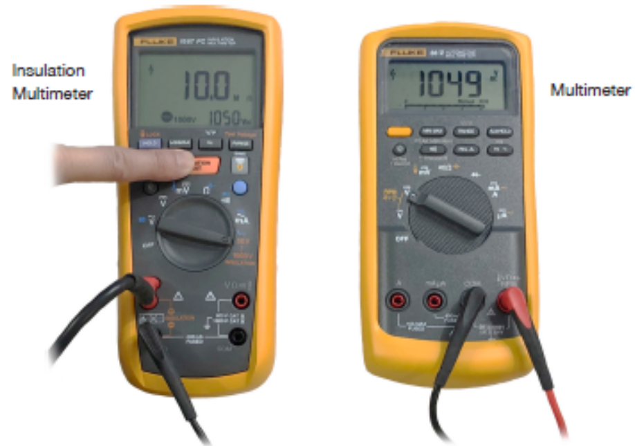
Figure 1-8, Verify Multimeter is Functioning Properly
