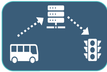
Figure 3. Centralized TSP Architecture
