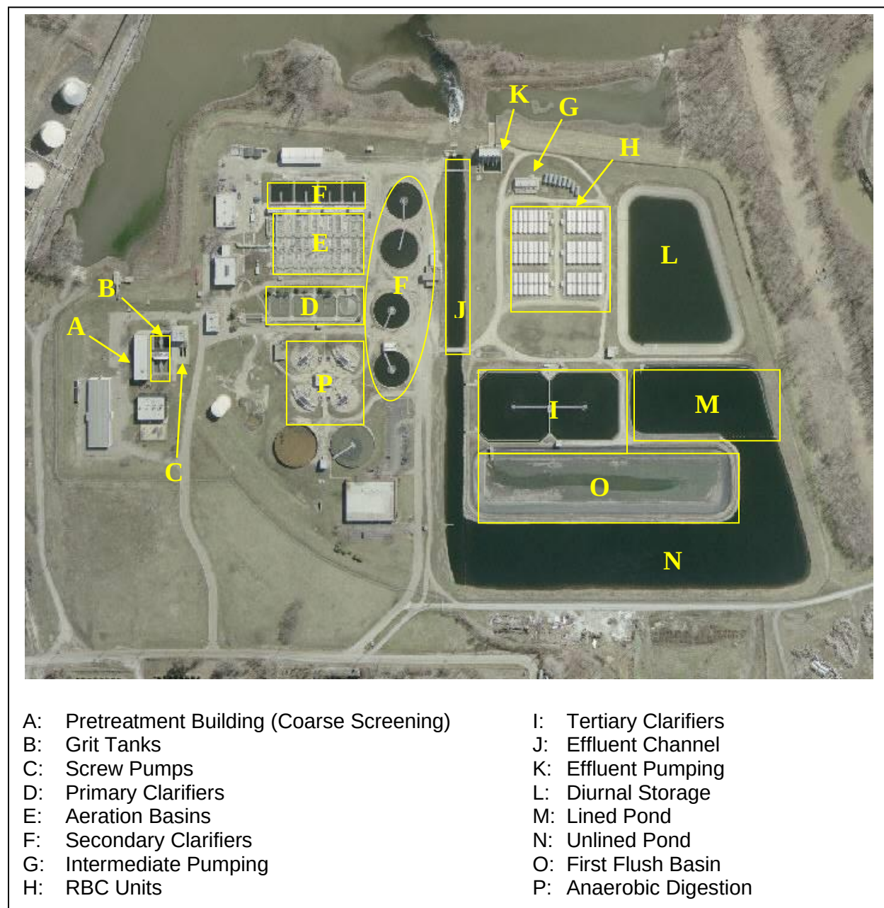
Figure 2-1 Greater Peoria Sanitary District Wastewater Treatment Plant and Treatment Processes
