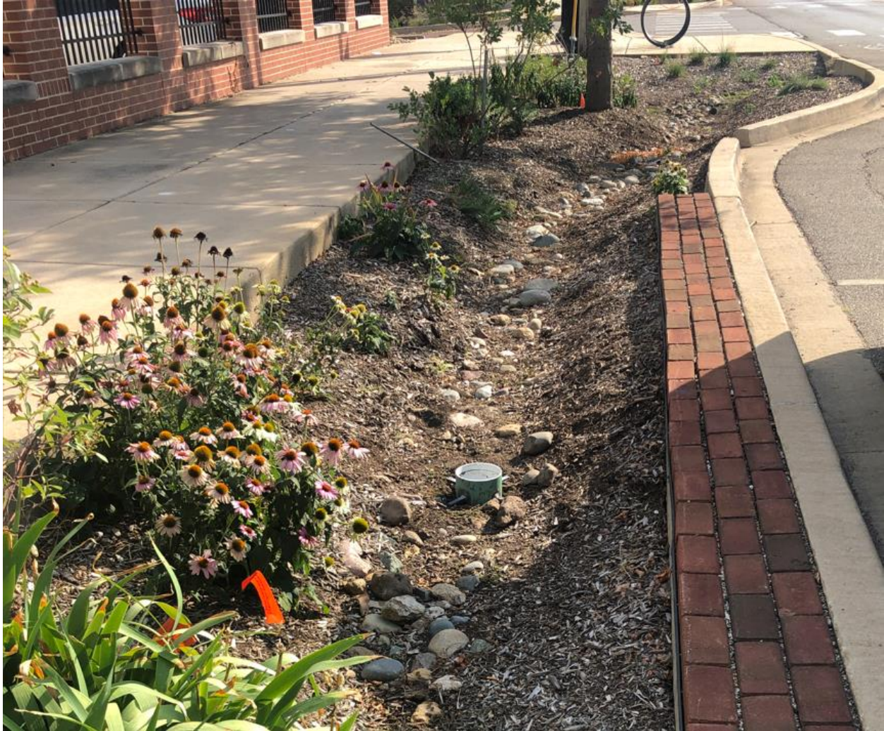
Figure 7 | Test Set Up for Single Ring Soil Infiltration Test of Peoria Bioswale
