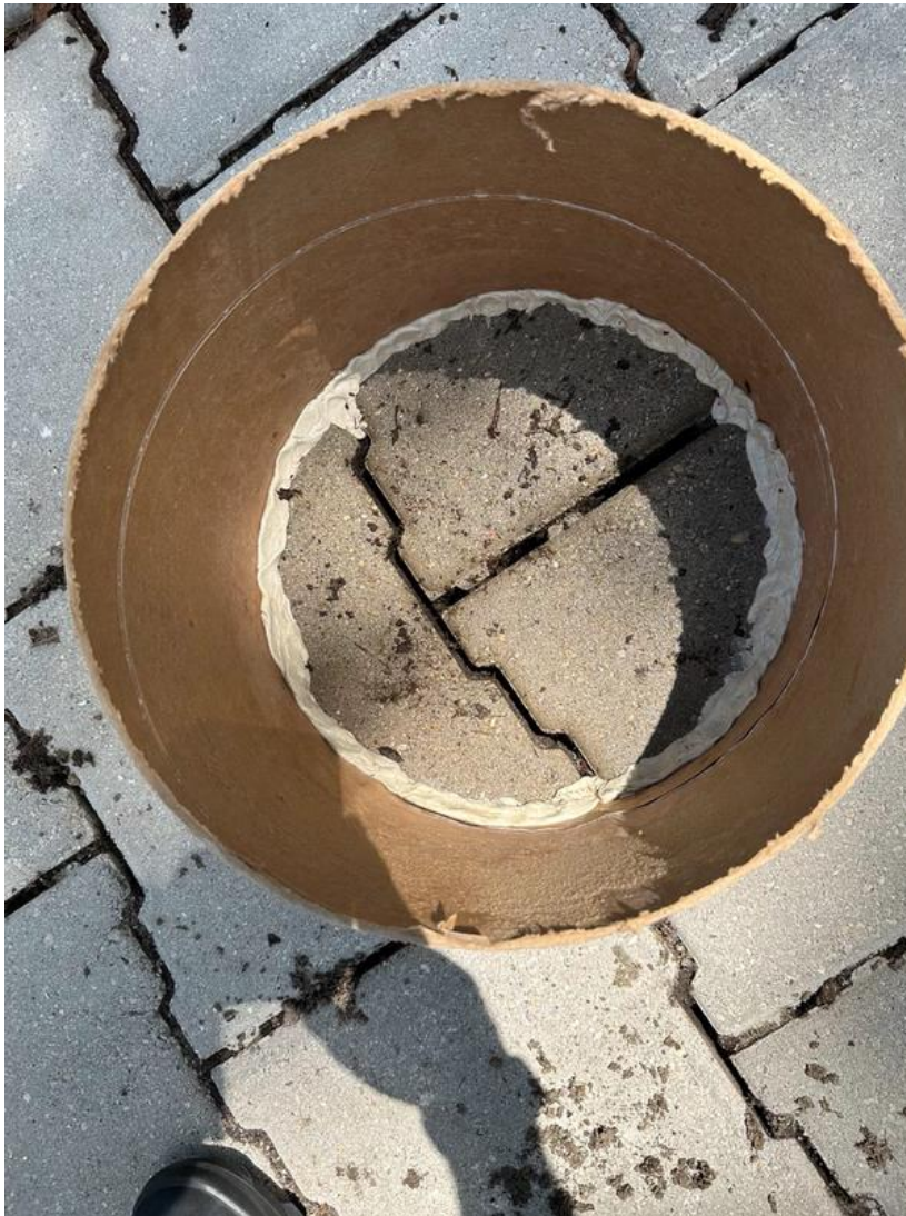
Figure 6 | Test Set Up Using ASTM C1781 for a Permeable Paver System in Peoria
