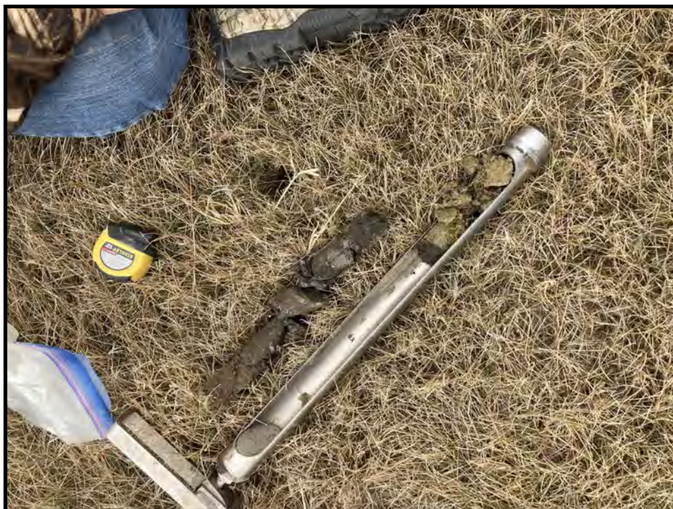
Photo 2. Upland 1 Point. View of the soils for the Upland point (Upl-1) for Wetland 1. The soil had salts present in the upper layer where mixing was present. The lighter layer present had a high value and chroma which characterized it as an upland soil. November 2, 2022.
